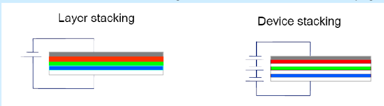
Fig. 2: White OLED in which different emitter layers are evaporated on top of each other in one device (left) and a so-called stacked device in which complete devices are evaporated on top of each other, connected by a special layer system (right). In the stacked device, each sub-unit emits in a different colour to create white emission.
